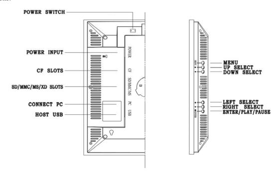
Insert one end of the power adapter into electrical outlet of the product and insert another end into AC electrical outlet up to standard.
